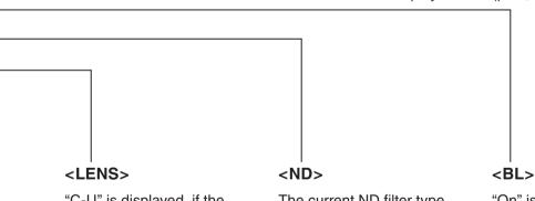
"C-U" is displayed, if the closeup lens is attached. If not, "Std" is displayed (p.43).
